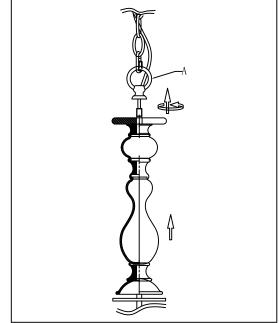
Step.1: Remove Top Loop (A) from fixture.
