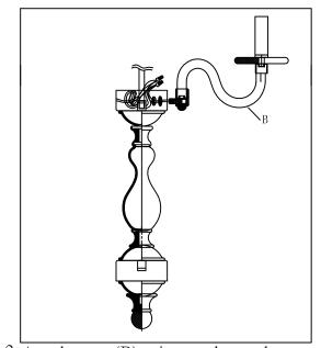
Step.2: Attach arms (B) using washer and nut provided. Then wire arm to the body of the fixture.
