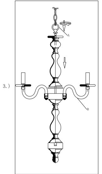
Step.2: Once all four arms (B) have been attached and wired, carefully secure upper half of fixture to central using Top Loop (A).
