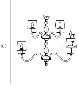
Step.8: Place shade (H) on candle cover and secure using screw ring provided. Then, install 40 Watt candelabra base bulb.
