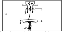
Step.5: Attach appropriate amount of chain to loop to achieve desired mounting height. Thread wire through every 3rd loop of chain. Remove ring from loop and slide down chain. Place canopy (B) onto chain and let slide to top of fixture. Install nipple and cross bar into top of chain loop. Wire fixture to wires in outlet box. Copper wire is for Ground. Pull canopy through screw ring (C) up chain to ceiling
