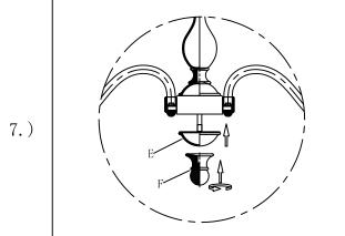
Step.7: Once all arms (G) are wired and secured, re-attach bottom cap (E) using finial (F).
