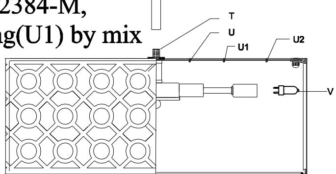
11. Hang the CRS22384-L, CRS22384-K to the metal ring(U2) by mix
